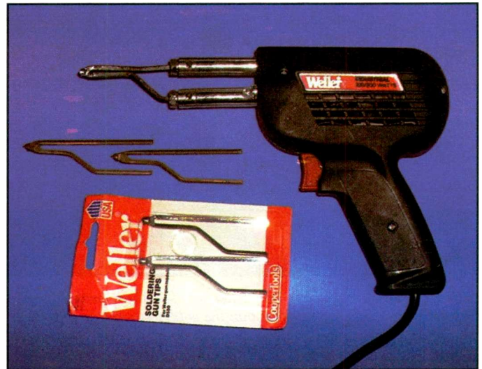
Photo B. This dual-wattage Weller gun is rated at 200 and 300 watts. The wattage is determined by two positions on the trigger. Two styles of replacement tips are shown: bare copper and plated.
