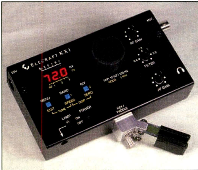
A nice close up of the Elecraft KX-1 CW transceiver, all tricked out with the internal automatic antenna tuner, the 30-meter option, and the ambidextrous paddles. This compact transceiver covers 40, 30, and 20 meters, CW only, and, using the internal Lithium Ion battery pack, is capable of 1.5 watts of RF output. If you happen to have 12 to 15 VDC available, the KX-1 can put out a maximum of 4 watts. All you need to add is a set of ear buds and an antenna. Nice little "doomsday radio" package, huh?
