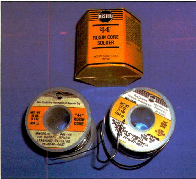
Photo A. Here are two one-pound rolls of Kester rosin core solder. One is a .031-inch diameter, too small for point-to-point wiring work, but ideal for printed circuit boards. The larger diameter solder is .062 inch and is the best size for working on vintage equipment.
